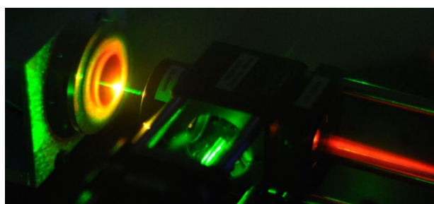
Fig.1: Spinning liquid crystal laser (left), capable of stable higher average power emission (red).
